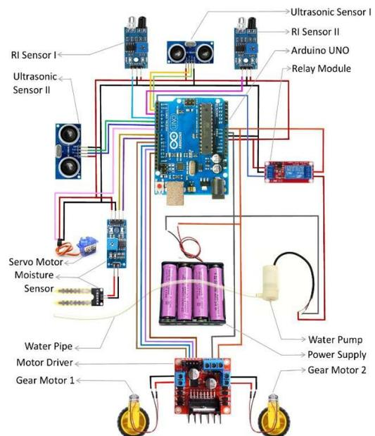
Fig. 4. Circuit Diagram of The System
