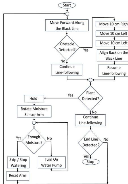
Fig. 3. Flowchart of the system's operation
