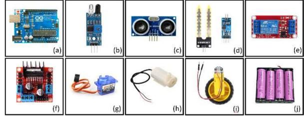
Fig. 1. Shows the (a) Arduino UNO, (b) IR Sensor, (c) Ultrasonic Sensor, (d) Soil Moisture Sensor, (e) Relay Module, (f) Motor Driver, (g) Servo Motor, (h) Water Pump, (i) Gear Motor, (j) Power Supply
