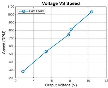
Fig.4: Voltage VS Speed Graph of a UC3843 PWM-Controlled Buck Converter for precise speed regulation of a DC Motor
