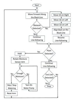
Fig. 3. Flowchart of the system's operation
